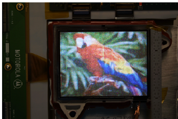
Video Image of a 4.6" diagonal NED prototype with 726 μm pixel size which represent a piece of a 16:9 63" (1920x1080) diagonal HDTV.
