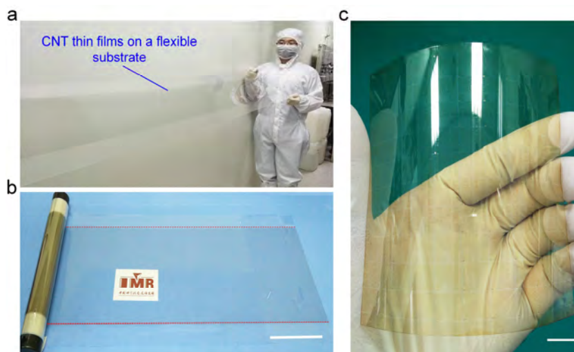
Fig.1 (a) A single-wall carbon nanotube (CNT) thin film on a flexible PET substrate with a length of more than 2 m. (b) A roll of uniform SWCNT thin film on the PET substrate (scale bar, 0.1 m). (c) Photograph of all-CNT thin film transistors and integrated circuits fabricated on a flexible PEN substrate with a size of 100 \times 100 \text{ mm}^2 (scale bar, 10 mm).
