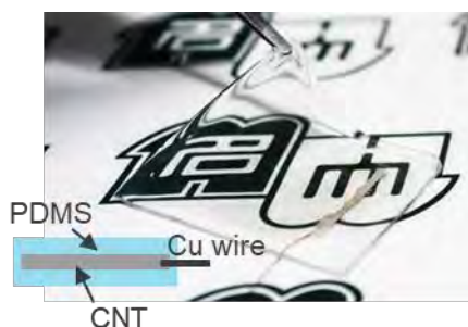
Fig. 1 Photograph of fabricated CNT TG. The inset is a schematic structure of the TG.
