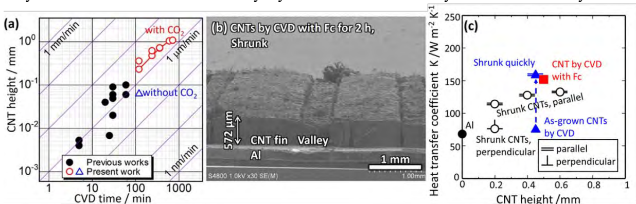
Fig. 1. (a) Heights of CNT arrays grown on Al substrates [1], (b) SEM of the CNT fins formed by ferrocene-assisted CVD without sputtered Fe catalyst, and (c) heat dissipation performance of Al with various CNT fins.
